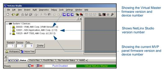
FIG. 37 NetLinx Workspace window (showing panel connection via a Virtual NetLinx Master)
